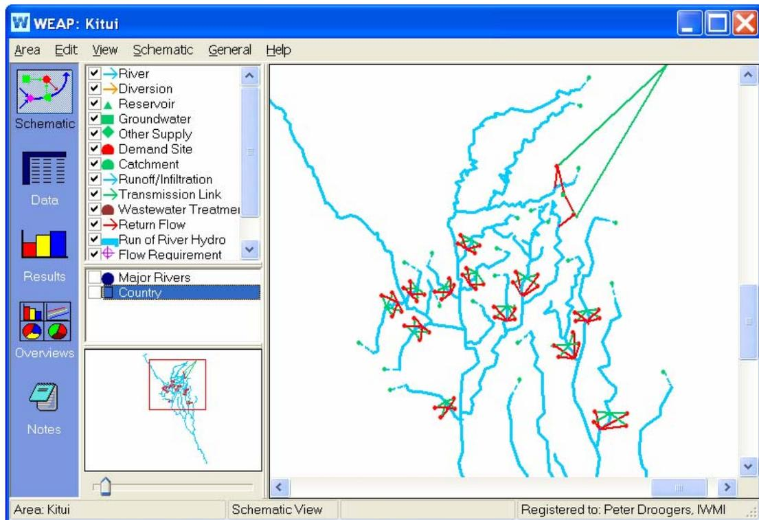
Figure 1. User interface of WEAP with on the left the five main views.
