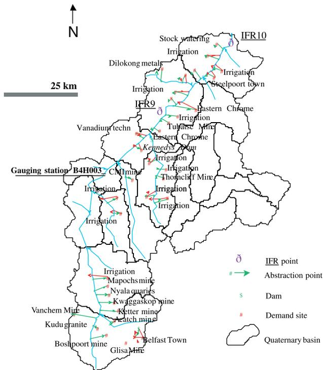
Fig. 2. Schematic representation of the Steelpoort basin for WEAP analysis showing quaternary basin sub-divisions and main abstractions.
