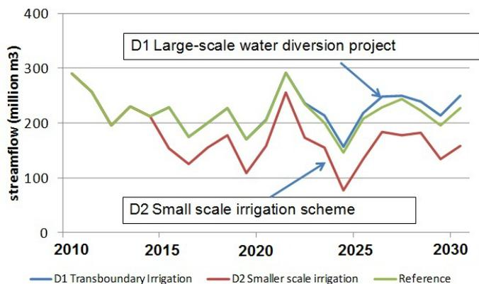
**Figure 26:** Outflow from WEAP simulated under two water resource development scenarios
