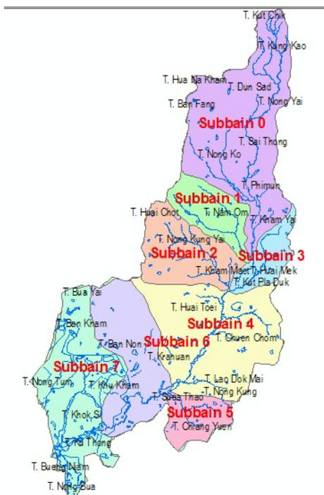
Figure 9: Map showing the configuration of the WEAP model to simulate flow within eight sub-basins (C00 to C07) of HSB basin used for the model calibration.
