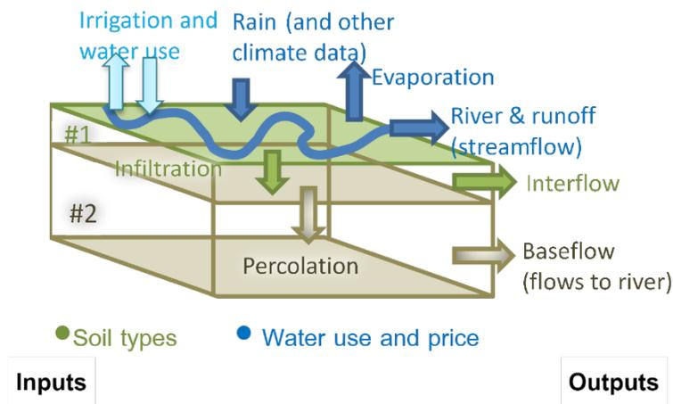
Figure 8: Schematic diagram of two-bucket model used in WEAP with some inputs and outputs
