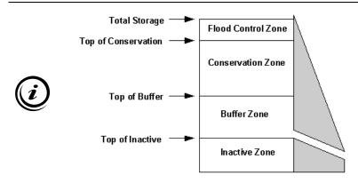
As illustrated by the figure to the left, WEAP allows the modeling of advanced reservoir operation through the definition of several zones that have different operational constraints.
