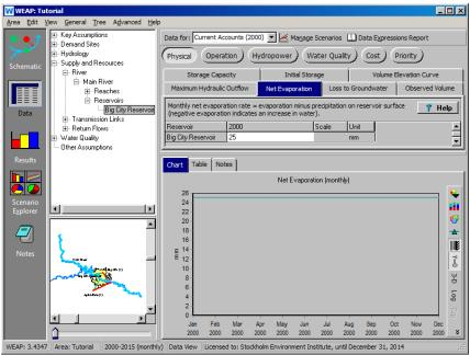
The "Volume Elevation Curve" is used both to model the surface for evaporation and to compute the head in case hydropower production is simulated. A cylindrical shape is assumed in converting reservoir volume and elevation into reservoir area.
