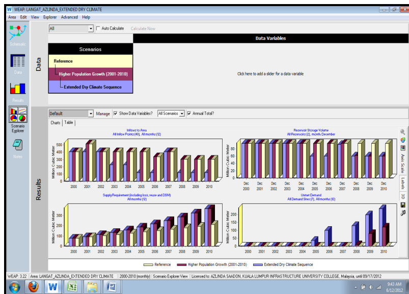
Figure 4.9: The Overall Result for Scenario 3: Extended Dry Climate Sequence in Comparison with the Scenario 1: Higher Population Growth (7%)
